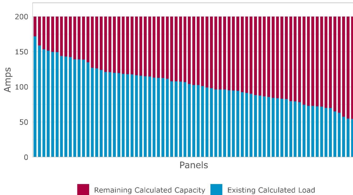
Figure 5. 200-amp Panel Existing Capacities. (n = 73). Source: Massachusetts RBUECS Study Phase 7.
